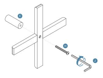
Attach 1 x pole (C) to assembled frame and secure with 1 x bolt (H). Tighten with an Allen Key (J).
