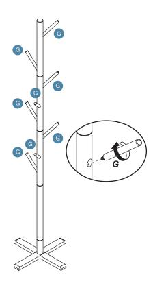
Attach 8 x pegs (G) into assembled frame as shown.
